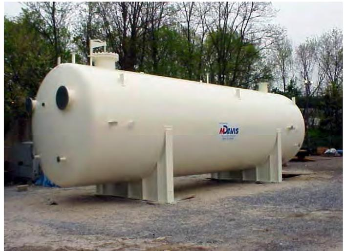
We also have design capabilities to perform alterations, which could include adding large nozzles, changing construction materials, or adding load-inducing components such as platforms. Our shops can fabricate the replacement components, and our field crews perform the welding to install right on our customer's site. We transport pressure vessels, heat exchangers, and components to our facilities to perform the repairs, then transport them back to the site, ready for use.
